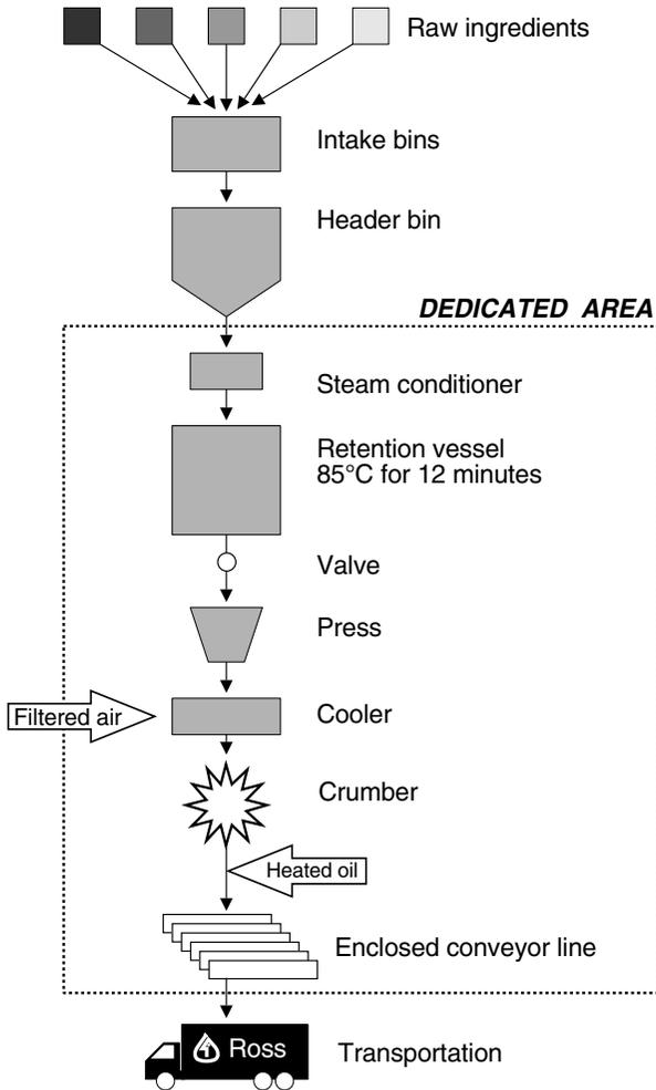
FIG 2: The diagrammatic layout of a dedicated poultry feed-mill
