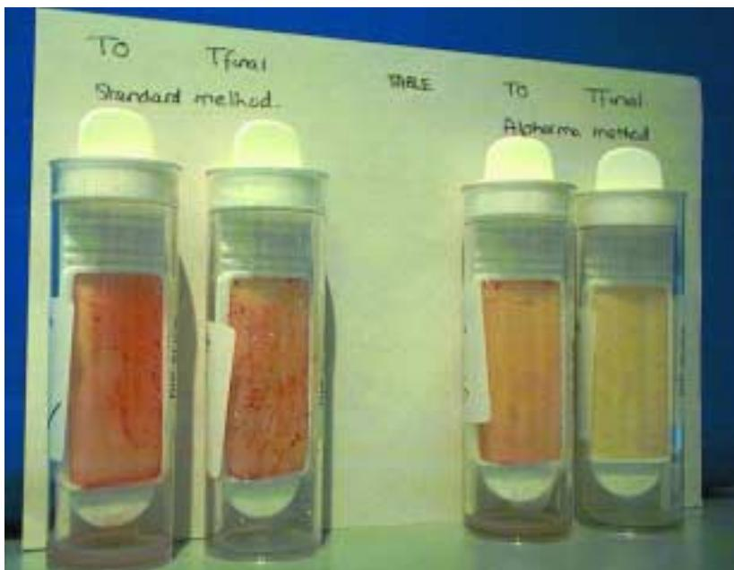
FIG 2: This shows a photograph of dipslides used to sample the vaccination table using the Control (here called Standard method) and the Test (here called Alpharma method) Treatments.
