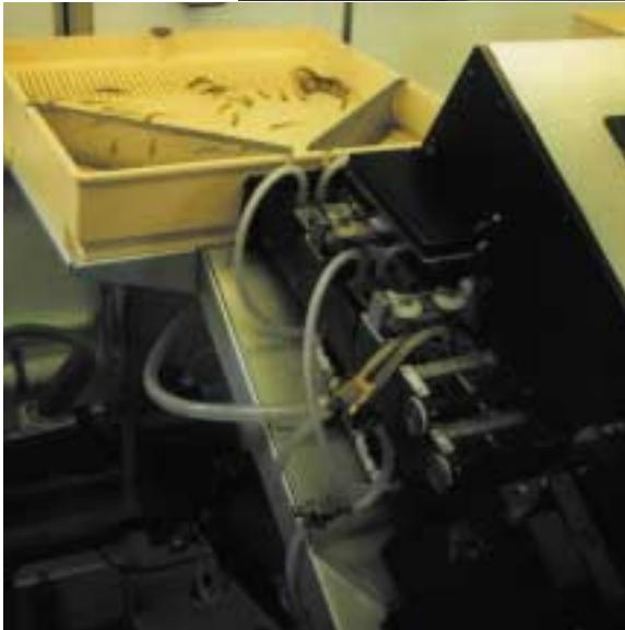
FIG 2: The volitional entry tray of a single line in a mass marking trailer. The fish are not anaesthetised and enter the tagging line through their own swimming action. Each line can tag, mark and vaccinate up to 2000 fish per hour.
