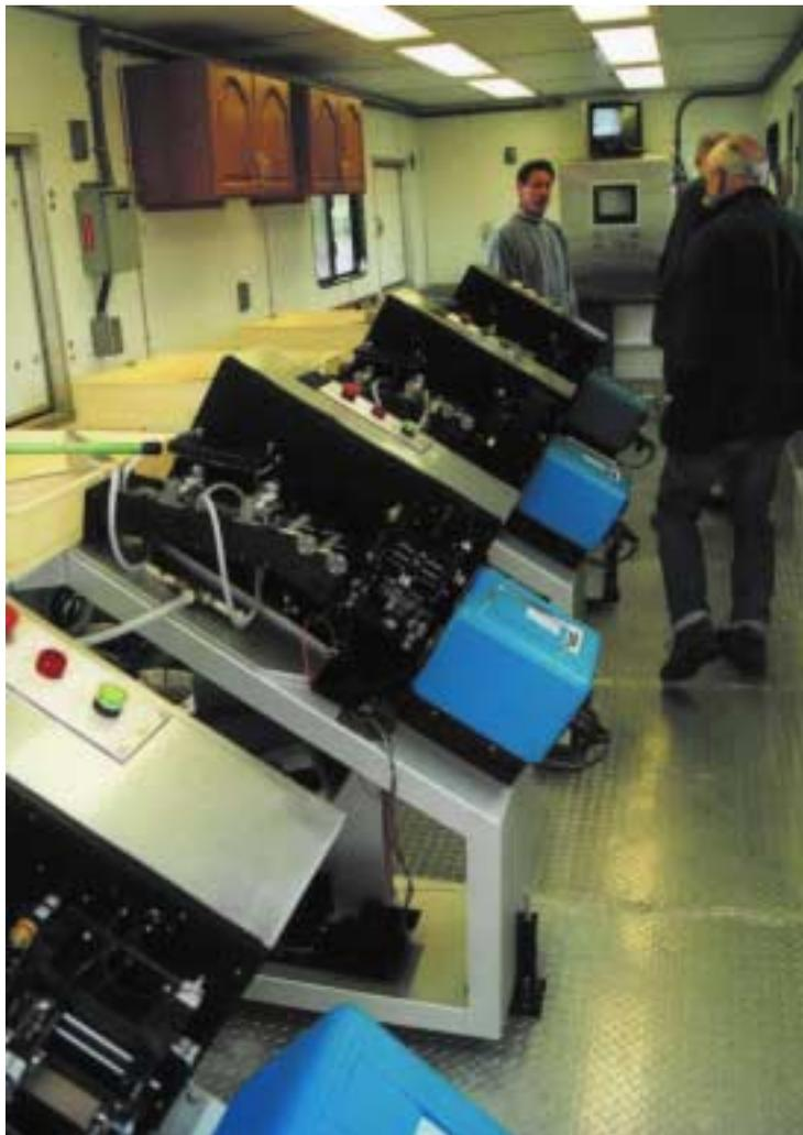
FIG 3: The interior of a mass marking trailer showing four tagging and marking lines.
